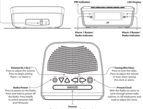
Press to snooze the alarm after it sounds. In on mode, press repeatedly to set the sleep timer.
